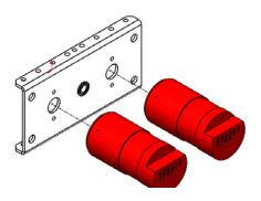
**Step 3**: Install six M3-0.5 x 6mm long socket head screws (am-1254) in each NeveRest motor to secure it to the gearbox plate.
