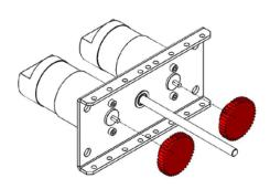
**Step 4**: Install the 6mm D-Shaft (am-3226-100) into the center bearing such that the end of the shaft is
