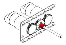
**Step 8**: Press a 6x12x4 Flanged Bearing (am-3377) into the center 12mm hole of a PicoBox Twin Turbo gearbox plate (am-3439).
