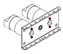
**Step 5**: Install two Pinion Assembly onto the NeveRest Motor shaft. Be sure to place the boss of the Gear against the motor. Tighten the #10-32 set screw to lock the Pinion Assembly in place.
