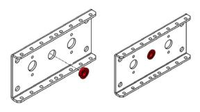
NOTE: Make sure the flange of the bearing is flush against the sheet metal of the gearbox plate.
