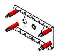
**Step 11**: Insert the Axle of the Gearbox Assembly into the bearing on the PicoBox Twin Turbo gearbox plate. Align the four 1/4-20 screws with the 1/4" holes on the PicoBox Twin Turbo gearbox plate is up against the Picobox Spacers.
